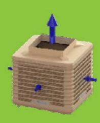
WetBoxes contain inbuilt evaporative cooling pads and should be used as part of a mechanical ventilation system or air handling solution with a paired supply and extract fan. They are designed to be externally mounted and the standard configuration is down flow, where air is supplied from the base of the cooler into the area that requires cooling.
