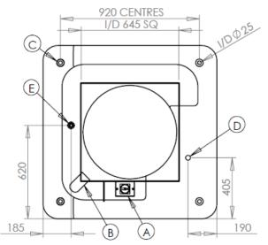
\*Note that all dimensions shown are nominal and have a ±10mm tolerance due to manufacturing processes employed.
