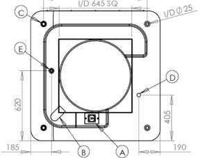
\*Note that all dimensions shown are nominal and have a ±10mm tolerance due to manufacturing processes employed.
