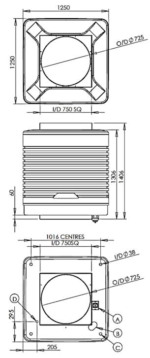
Note that all dimensions shown are nominal and have a ±10mm tolerance due to manufacturing processes employed.
