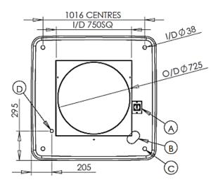
Note that all dimensions shown are nominal and have a ±10mm tolerance due to manufacturing processes employed.
