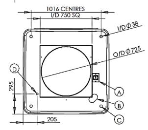
Note that all dimensions shown are nominal and have a  $\pm 10$ mm tolerance due to manufacturing processes employed.
